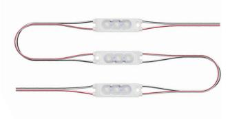
The BackLED Eco M Plus family features a Flat Ray lens to provide a uniform beam distribution on the face of channel letters that are 4" to 5" deep. The 6500K color temperature provides the crisp white light that has become the standard in the signage industry.
