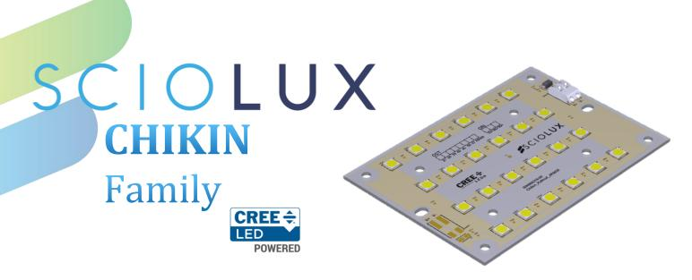
CHIKIN module based on CREE LED technology, J Series 5050 family, provide us with exceptional efficiency at a competitive cost, breaking the barriers between medium and high-power technology.
