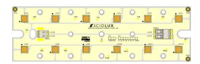
BALAM module based on the technology of the CREE LEDs, J Series 5050 family, give us exceptional efficiency at a competitive cost, breaking the barriers between medium and high-power technology.
